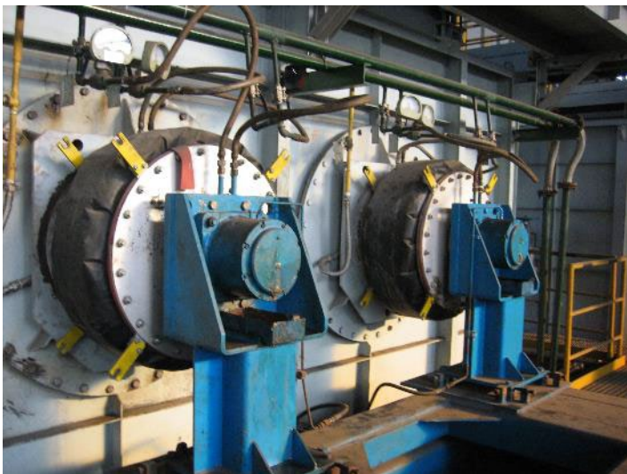
Fabric expansion joints compensate for the movements of the steering rolls that centrally guide the sheet metal bands through the furnace. Image: ©Frenzelit GmbH
